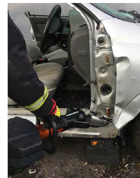
STEP 2 After blocking under both the A and B posts, make a relief cut in base of A post. Generally and on saloon cars this would be horizontally and just underneath the reinforced structure of the lower hinge. This positioning may need to be adapted on larger vehicle structures to allow for effective tip positioning and lifting
