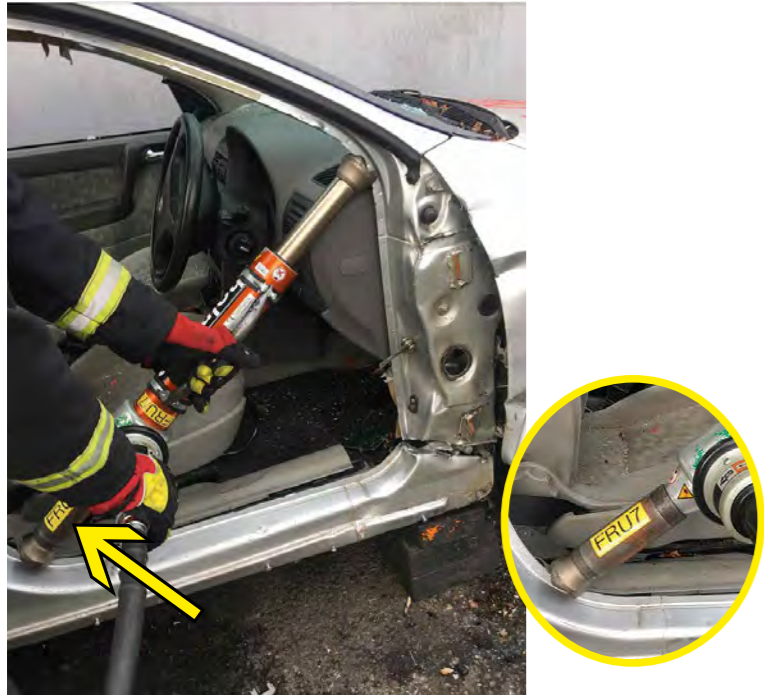
STEP 3: Insert the stationary ram base into the junction of the floor edge with the B post. Extend the ram arm until its head engages with base of the A windscreen post Note that a short extension piece has been attached to the ram base for the initial ram arm extension, in order to fit within the initially available space.
